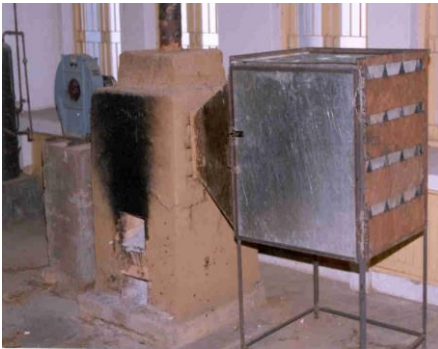
Waste fired dryer
